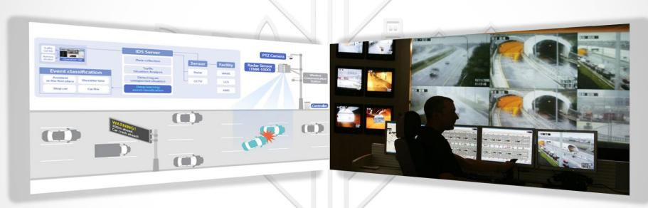
This system is aimed at monitoring and controlling incidents of urban and road tunnels, which works by using closed-circuit cameras embedded in the tunnels. The automatic accident detection system of this system can detect the desired incidents and behaviors by using the images obtained from closed-circuit cameras and report the warning to the officials and personnel of the tunnels.
